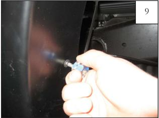
Using #2 Phillips Screwdriver, insert a supplied Truss-Head Screw through existing holes in flare and into holes in clips (4 places).
