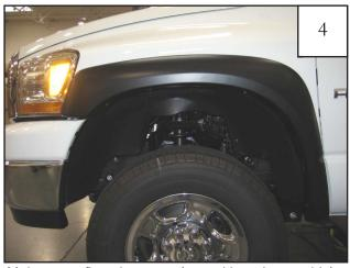
Make sure flare is correctly positioned on vehicle. Tighten all screws.
