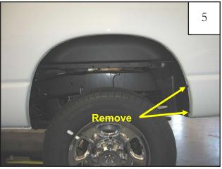
Using an 8mm socket, remove two factory screws from rear of wheel well. Retain for future use.
