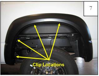
Slide a supplied clip over fender lip, aligning with existing holes in fender flare (4 places).
